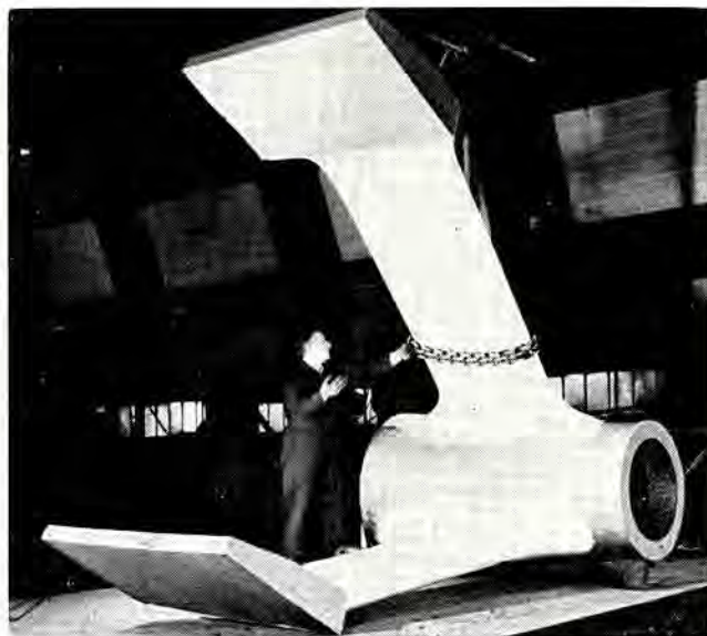
Cast steel A-bracket for Type 21 frigate
