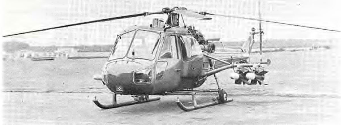
The Westland "Scout" helicopter fitted with Nord (now SNIAS) SS.11 wire-guided missiles and the Avimo-Ferranti AF.120 Stabilised Sight. The Sight's rotatable head can be seen projecting through the helicopter's canopy
