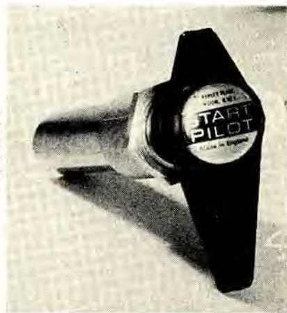
Fig. 2. The pump unit which is installed at the 'control centre'
