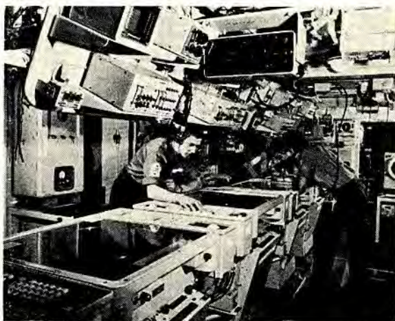
The operations room of HMS 'Torquay' with the CAAIS system installed. Members of the 'Torquay's' crew are seen at the display units associated with the system
