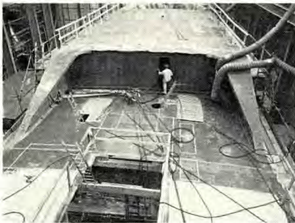
Most of the decking complete, together with the break-of-forecastle moulding
