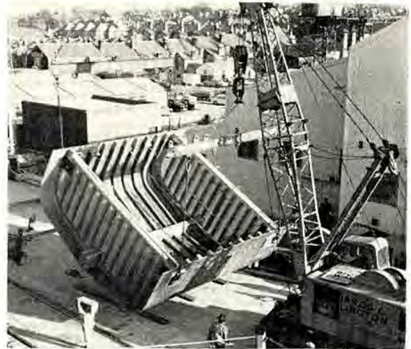
The second glass-reinforced plastics structural test specimen completed in November 1968. The form of construction seen here is basically that which has been chosen for the complete mine-hunter prototype
