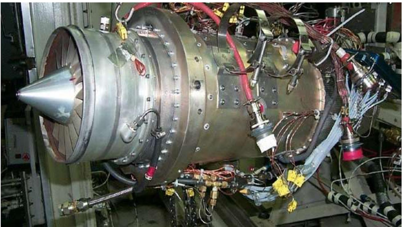
engine. The engine contains an Ultra Compact Combustor (UCC) that was developed to improve combustion efficiency, stability and ignition without sacrificing performance. It is also 69% smaller in volume than the original UCC.
