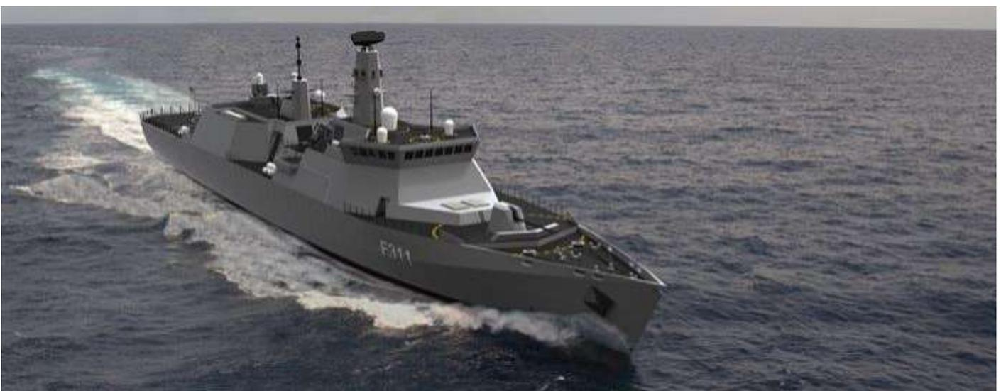
The Nodal Modular Physical Architecture (NMPA) approach to the design allows for configurable options. Each node has the ability to accept different systems; for example a customer may wish to have a simple 30mm Small Calibre Gun system in place of the forward Mk41 Vertical Launch System (VLS), or place a SeaRAM or Phalanx in this position. Future capability growth would be enabled by space, electrical power and weight margins.
