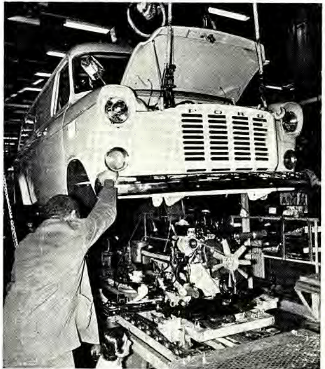
Ford Transit body shell being lowered above the 2.4-litre diesel power unit at the commercial vehicle plant at Langley, Bucks
