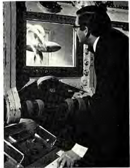
A propeller model on test showing cavitation from the blades
