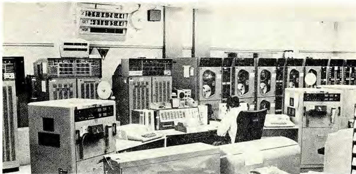
From left two Univac 642B computers with an expanded memory unit between. In the centre right are eight tape transports fully duplexed with the 642B computers. To the right are two Univac 1218 computers and associated magnetic tape unit with two tape transports. In the foreground are the I/O consoles and the operator's monitoring position
