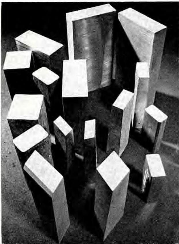
Fig. 1. Some of the various extruded blade blanks made by Henry Wiggin in Nimonic alloys for gas turbine manufacturers
