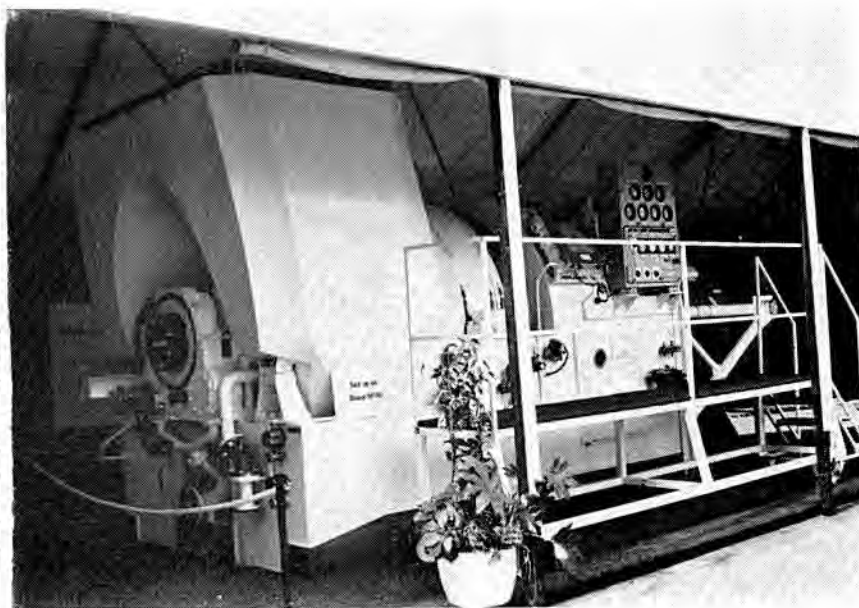
Rolls-Royce Marine Olympus gas turbine package, ordered as the boost engine of the Royal Navy's Type 42 destroyers and Type 21 frigates, for vessels of the Royal Netherlands and Argentine Navies and nominated by the Royal Australian Navy
