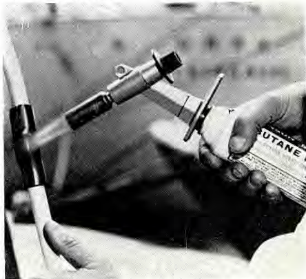
Ampsulation tubing being reduced to size by heat from a butane gas torch
