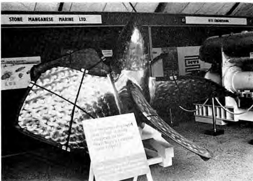
Stone Manganese Marine five-bladed propeller for a 'Leander'-class frigate. The 'cropped' blades of this highly efficient design contrast interestingly with merchant vessel practice. SMM will supply their Mark XX cpp's for the frigate and destroyer programmes of the Royal Navy
