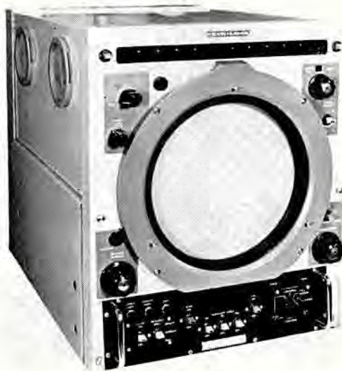
The Type 1006 Naval radar which was developed by Kelvin Hughes will be the Royal Navy's standard navigational radar in the seventies
