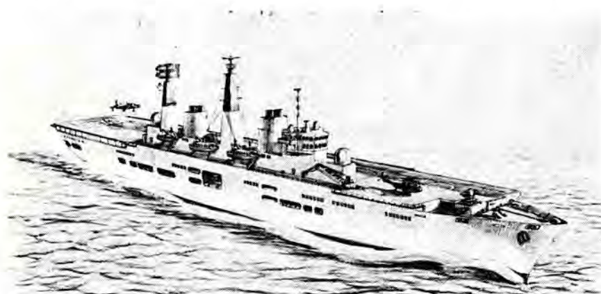
Projected 'through deck' cruiser for the Royal Navy—largest all gas turbine-powered naval ship
